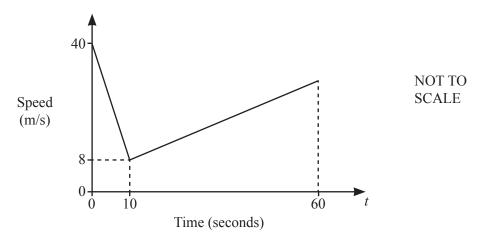
The train slows down uniformly from a speed of 40 m/s to a speed of 8 m/s in a time of 10 seconds. It then accelerates uniformly during the next 50 seconds.
